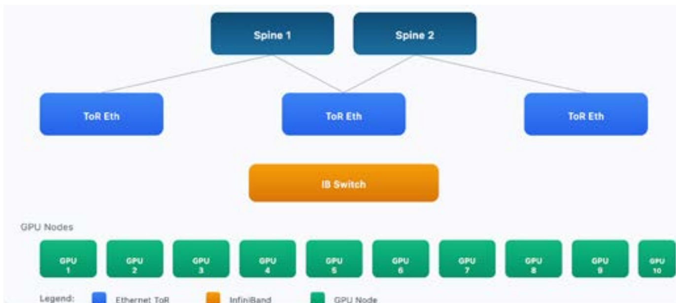
Exhibit 9: Rack-level deployment topology with dual-fabric architecture
